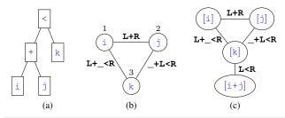
Figure 5. (a) the AST of expression i+j < k, and two dependency networks built from the AST relations: (b) for name predictions, and (c) for type predictions.
