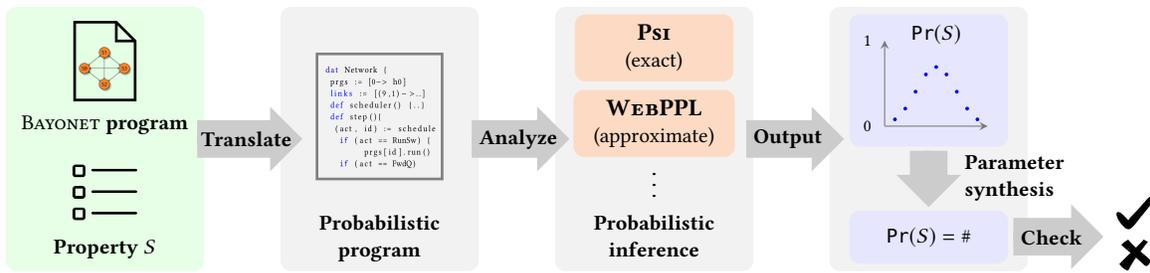
Figure 1. Probabilistic Inference for Networks with BAYONET.
